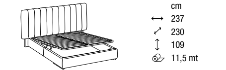
DTMFBX3 DOUBLE BED WITH FLOOR STANDING BED FRAME FOR 180X200 WOODEN SLAT SYSTEM WITH SCISSOR-LIFT MECHANISM
